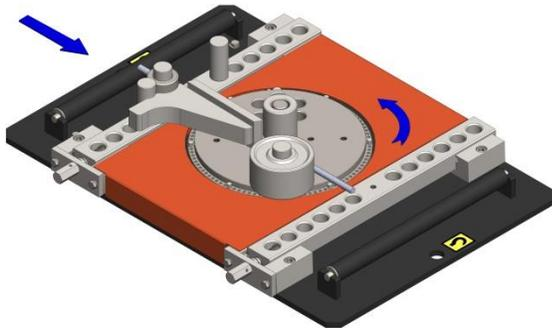
Fixing the rebar to be bent on the machine with the help of bending sleeves (4b)
