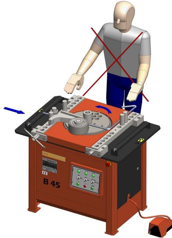
**Figure 7:** Wrong positioning of the person making bend
