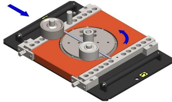
Fixing the rebar to be bent (4a) on the machine in multi-rebar bending with the help of a retainer (4c)
