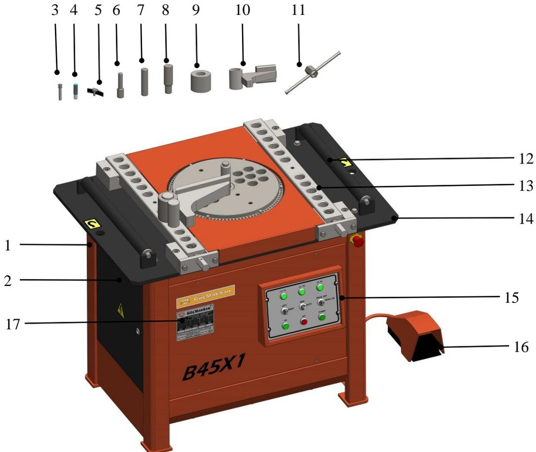
**Figure 1:** Main parts of bending machine
