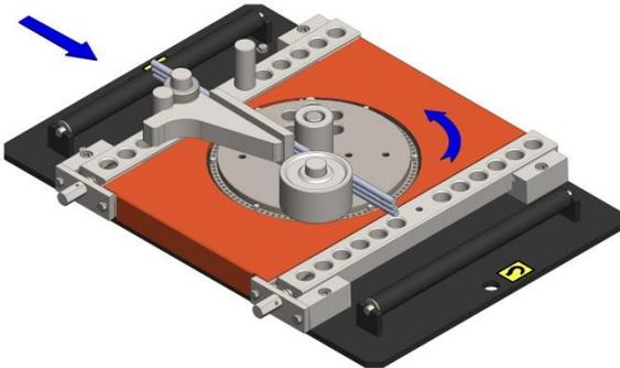
Fixing the rebar to be bent (4b) on the machine in multi-rebar bending with the help of bending sleeves. (4d)
