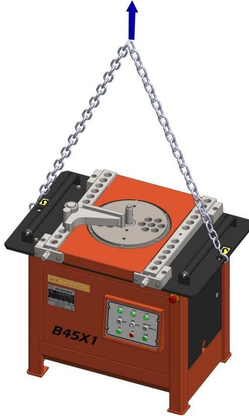
**Figure 8:** Handling the machine
